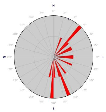
Fig. 9: A Rose Diagram showing dip direction within the study area
